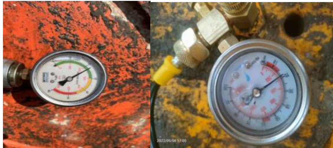
1) Before the excavator's confluence, the pressure is 22MPa, and the nitrogen pressure is 1.8MPa (as shown in the diagram below).
